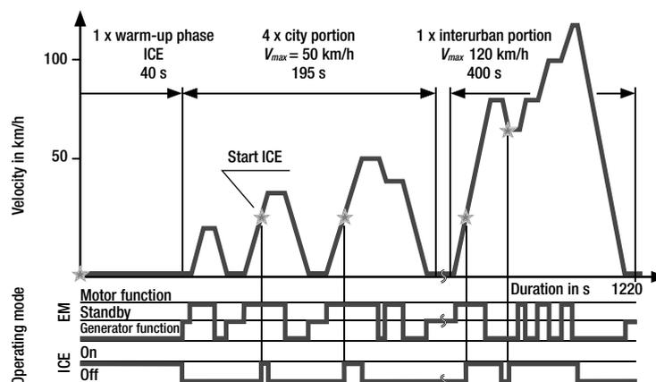
Figure 2: Representation of Signals for the Hybrid Drive Including Internal Combustion Engine (ICE) and Electric Motor (EM)
