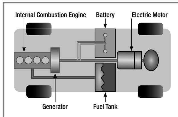
Figure 1: Components Included in a Serial Hybrid Vehicle
