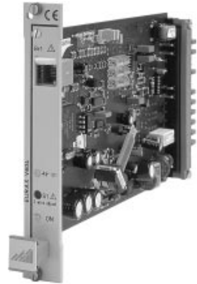
Fig. 1. Transmitter EURAX V 604, front plate width 4 TE.
