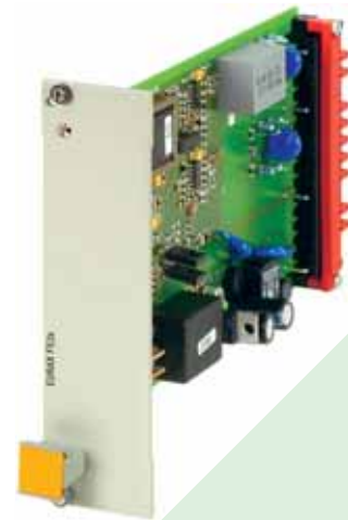
Fig. 1. EURAX G 537 as plug-in module for 19" rack-mounted case, front plate width 7 TE.
